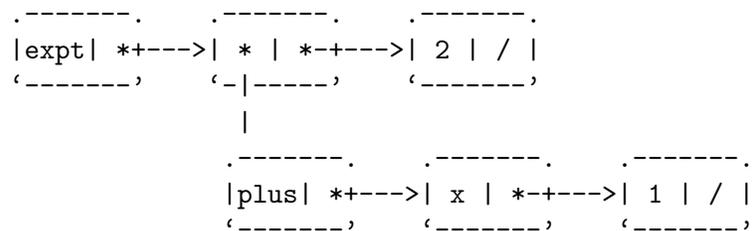
In this graph the `cars` contain the symbols or numbers or they point to substructures (downwards) while the `cdrs` point to the successors (to the right) until the end is reached.
